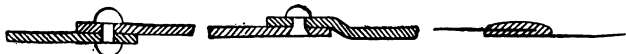
FIG. 172. A Riveted Lap Seam for Plate. FIG. 173. Flush Riveted Lap Seam. FIG. 174. Soldered Lap Seam.
